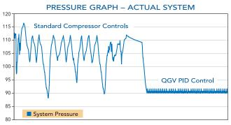
The Quincy QGV delivers constant pressure within 2 psi at part load capacities as low as 15% – nearly 20% lower than the industry standard.
