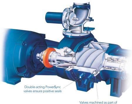
Valves machined as part of housing to prevent blow-by efficiency losses
