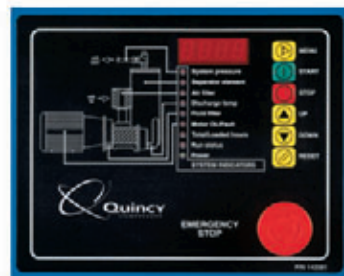
Microprocessor-based electronic control efficiently manages compressor supply to match system demand.
